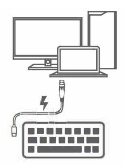
Wired mode, plug the keyboard to PC by USB-C cable in the packaging.
