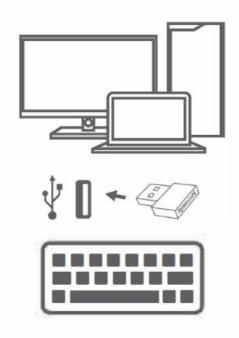
Put the mode switch to 2.4G (BT/2.4G/ OFF), Long press FN+R for 3 seconds, plug the USB dongle to PC USB port, PC will detect to keyboard.
