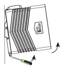
Remove the switch from the standard 35mm DIN rail as shown in the diagram above.
