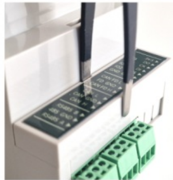
Figure 3: Opening the connector covers
