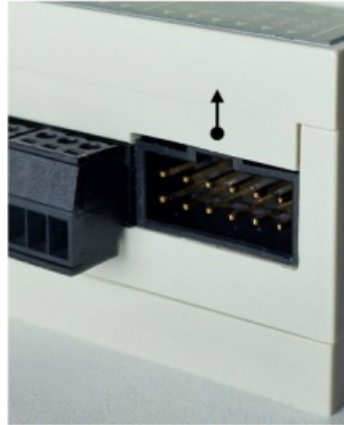
Figure 4: GPIO header location and pinout
