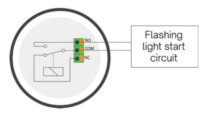
The BlackMax comes with a pre-wired orange light that begins flashing when the state-of-charge (SOC) of the battery drops to 20% or the battery voltage drops below 51 volts, whichever comes first.
