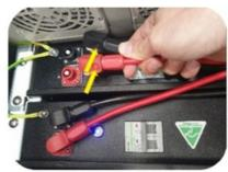
Remove the battery cables by pressing the button on the side of the terminal and pull it straight up. **NOTE**: When installing the battery cable, simply push it onto the terminal until you hear a click.
