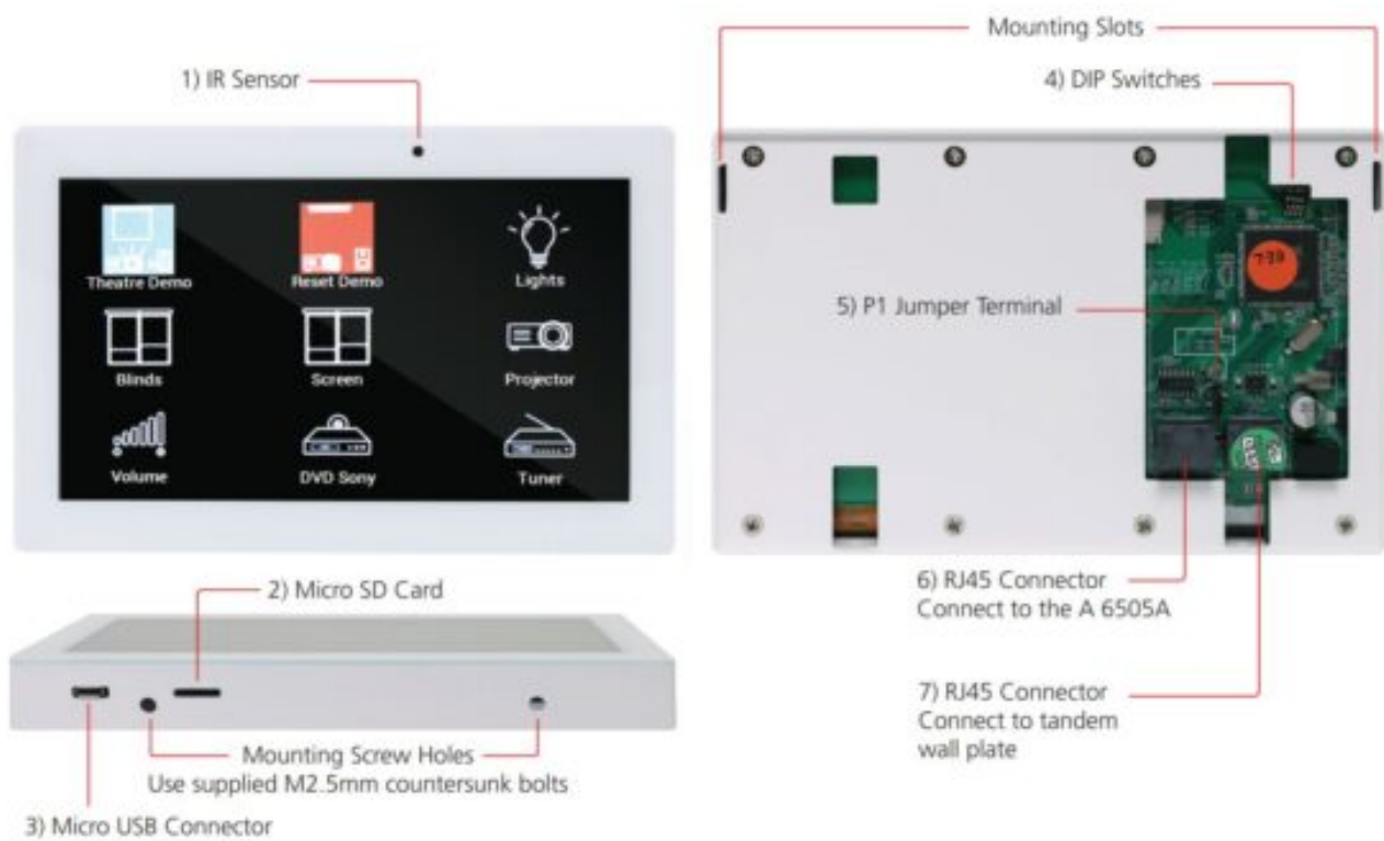
Fig 2.1a A6530 and A 6531 connections
