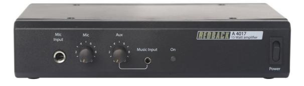
The A 4017 is a 15 Watt amplifier designed to operate on 12V DC, making it suitable for use in vehicles. It has a Mic input, Aux input and Music input, along with speaker output and a headphone output. The amplifier is internally protected by polyswitches which disconnect the speaker line when over-driven. It also features DIP switches that set the phantom power to the microphone input and adjust the Aux input sensitivity.
