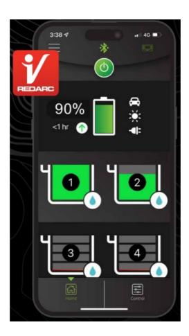
remote access to functions and information about the Red Vision compatible devices in your system. It includes battery level monitoring, system and input source monitoring, system diagnostics and firmware update notifications.
