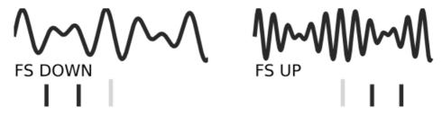
Start from the ring mod setting in the diagram. The RING MOD / FREQ SHIFT control adjusts the levels of the upper and lower sidebands, to blend between frequency shifting and ring modulation.
