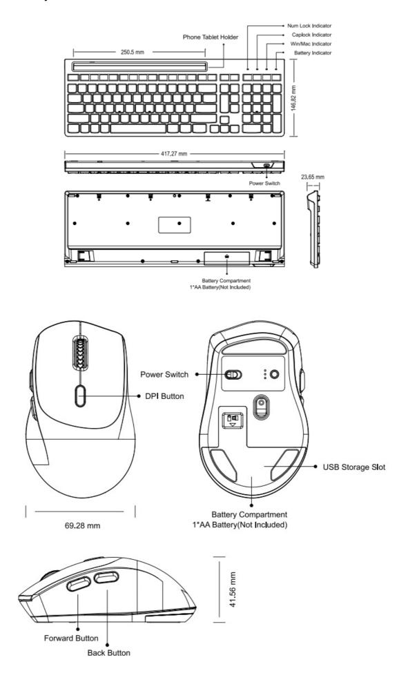
Step One: Take out the USB receiver on the bottom of the mouse, then insert to the computer. Open the battery cover, install an AA battery according the polarity mark in the battery box.
