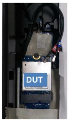
Remove 2 external Wi-Fi Antennas from the Wireless PCle NGFF2230 moduke board and remove the Wireless PCle NGFF2230 module board from PCle NGFF2230 connector port
