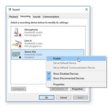
**Step 4:**Now you can access the HD Audio Manager to configure Stereo Mix and use Voice Recorder to record the sound.
