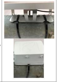
Plug the solar panel cable into the Data Gateway with the latch chip on t he top side as shown. This will turn the Data Gateway on. The status LE D will flash multi-colored when first turns on.
