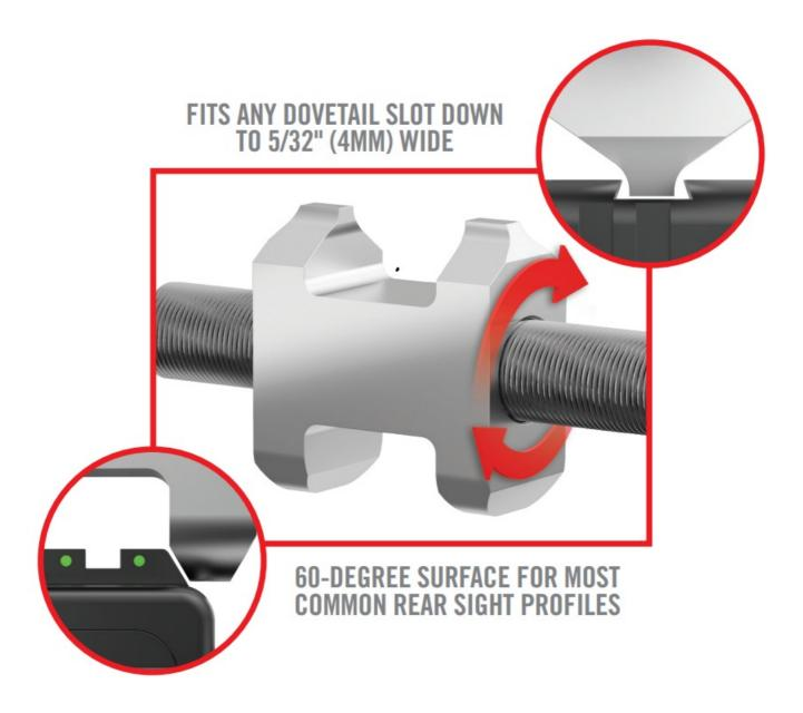
If you have a low-profile sight, or one with a small surface to push on, it is recommended to use the 4mm wide tooth side of the Reversible Press Block. This narrow tooth can reach down inside most dovetails, in order to align the Press Block as low as possible to the sight for maximum leverage.
