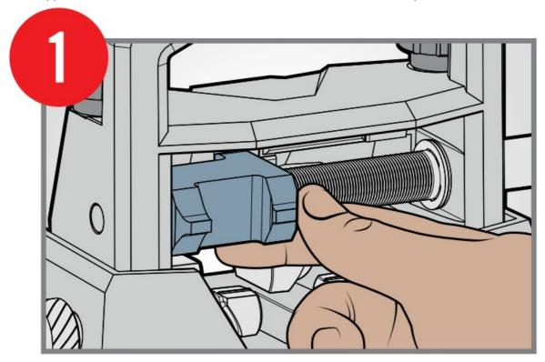
• Align clamp guidelines with center of dovetail slot and secure slide in cradle.
