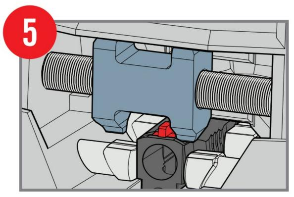
$\bullet~$  Turn Easy Torque Handle  $^{\text{TM}}$  and push sight through dovetail slot
