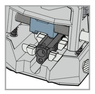
Loosen the two vertical frame bolts to allow for height clearance and help with visibility. Be sure to check the vertical stabilizer, to make sure it is up all the way. Mount pistol slide into slide frame.
