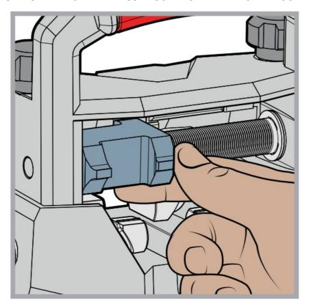
Select appropriate Reversible Press Block orientation. If you would like to use the opposite surface on the Press Block, rotate the crank clockwise to transport the Press Block all the way to the left. At this point, the Press Block should rotate freely without the support wall behind it. With the correct side selected, return the Press Block to the center by rotating the Easy Torque Handle<sup>TM</sup> counter-clockwise.
