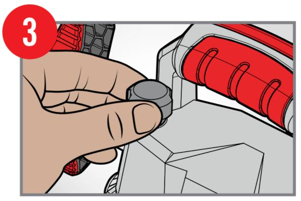
• Snugly tighten vertical stabilizer to hold pistol slide in place.
