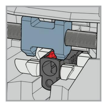
Use this step to ensure everything has remained aligned during the locking process and that the press block remains in correct alignment with the sight or dovetail slot and completely clears the slide to prevent damage. Special Note: when utilizing the 4mm tooth surface to push within the dovetail slot use extreme caution when lowering the Reversible Press Block down to this height. It is very easy to misalign features and cause damage to your gun's slide.
