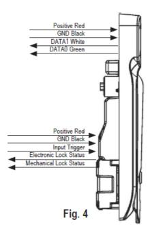
The reader modules of the swinghandle is accessed with a four pin connector attached to a harness connected to the module's circuit board. The module's connector pinout is:
