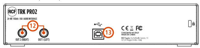
12. MONITOR BALANCED OUTPUT JACKS This output accepts a 6.35mm jack plug for the connection of active speakers or speaker amplifier input. 13 USB TYPE B PORT It provides the computer connection for data transmission and power supply.
