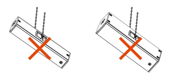
WARNING: Never suspend this speaker by its handles. Handles are intended for transportation, not for rigging.
