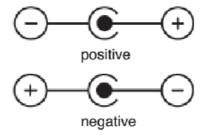
**Note:** Polarity information may be found next to the DC jack, user manual, or device information plate. The adapter plug tips have a positive (+) symbol on one side and a negative (-) symbol on the other side. The AC adapter receptacle says "TIP" on one side.
