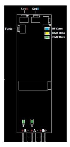
Dimmers don't have to be sequential. You can use RC4 OneTouch™ with the Set buttons for each individual dimmer. For example, if you want DimB to be set to DMX address 11, bring up 11 @ 30% (for the LED curve) at the board and press the SetB button. Remember: SetA assigns the 2 dimmers sequentially. The other Set button works individually. Always use SetA first.
