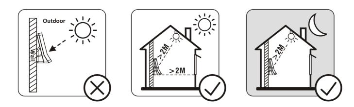
When installing outdoors, direct sunlight equipment, oblique sunlight equipment, or direct sunlight equipment through windows are prohibited When installing indoors, make sure that the place must be installed away from windows/doors / lamp more than 2 meters away equipment
