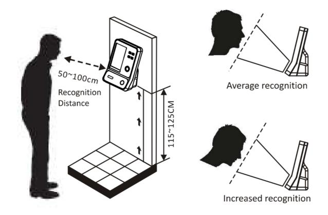
The installation height is mainly for shorter person Recognition distance is about 50~100cm Recommended installation height from the bottom of the machine to the ground is about 115-125cm Please bow your head slightly when recognizing to improve the recognition success rate
