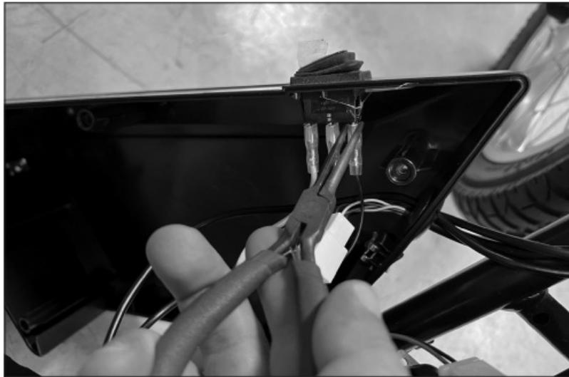
When re-connecting the controller to the power switch, make sure you connect the black wire to the gold-colored prong, the red wire to the middle silver-colored prong, and the yellow wire to the remaining silver-colored prong.
