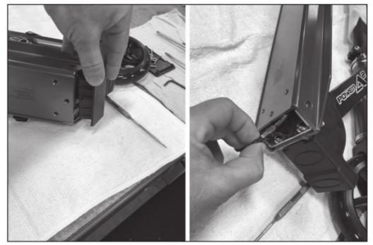
**Step 4**Remove the grommet from the metal bracket. Push the throttle wire inside the opening.
