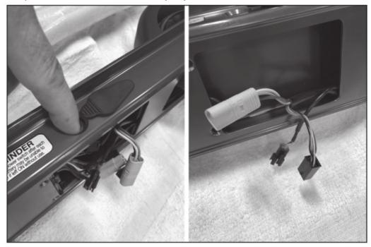
**Step 9**Disconnect the rest of the wires from controller. Remove and replace with new unit.
