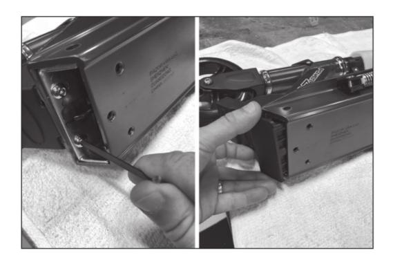
**Step 15** Reposition controller cover and secure with screws.
