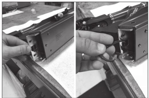
**Step 13**Reconnect throttle to controller and place the grommet back into the bracket.
