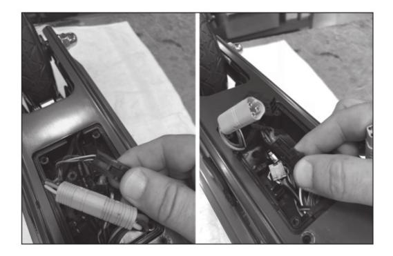
**Step 8**Push down on the power switch and slide the battery tray out of the deck.
