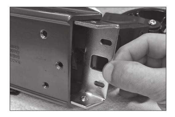
**Step 6**Remove the controller cover to access the wires.
