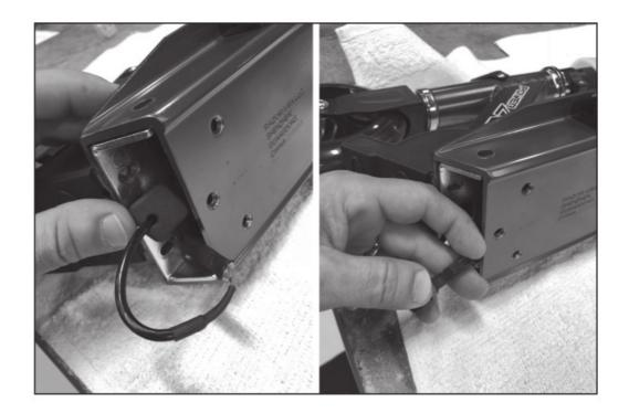
**Step 14**Secure the bracket to frame. Place the plastic cover back onto the unit.
