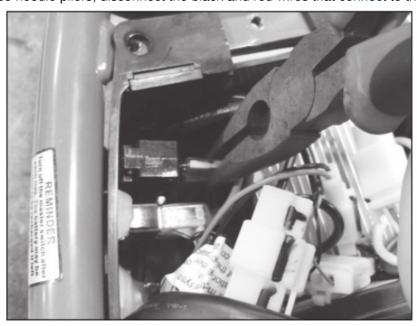
Step 7 Using long-nose needle pliers, disconnect the ring that holds the reset button to the battery tray.
