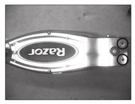
**Step 3** Using a 4 mm Allen wrench, remove the two (2) hexagonal screws on the deck cover. The locations of the screws are circled in the image below. Remove the deck cover and set it aside.
