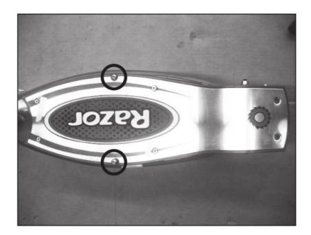
**Step 4** Using a Phillips screwdriver, remove the four (4) screws on the battery holder. Locations of the screws are circled in the image below. Remove battery holder and set aside.
