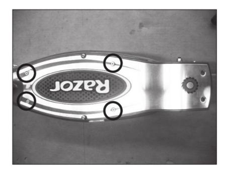
**Step 2** Using a Phillips screwdriver and an 8 mm wrench, remove the two (2) nuts and screws on the tail of the deck cover.
