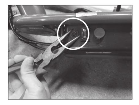
Step 8 Remove the reset button from the battery tray.
