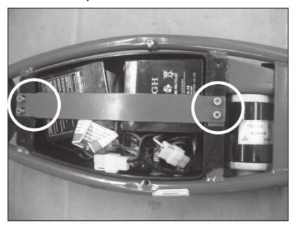
**Step 5** Locate and disconnect the battery from the controller before trying to disconnect the reset button.
