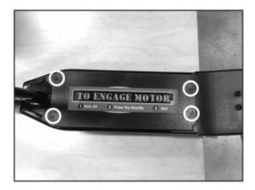
**Step 2**Using a Phillips screwdriver, remove the two (2) screws on the battery holder (circled in the image below). Remove battery holder and set aside.
