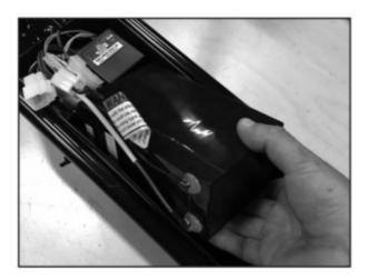
**Step 5**Using a Phillips screwdriver, remove the two (2) screws that attach the controller to the tray (circled in the image below). Remove old/damaged controller.
