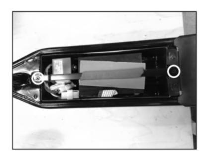
**Step 3**Disconnect all connectors from the controller.
