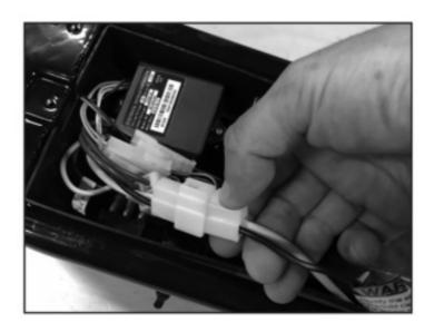
**Step 4**Remove the battery from the tray to give you access to the controller. Set battery aside.
