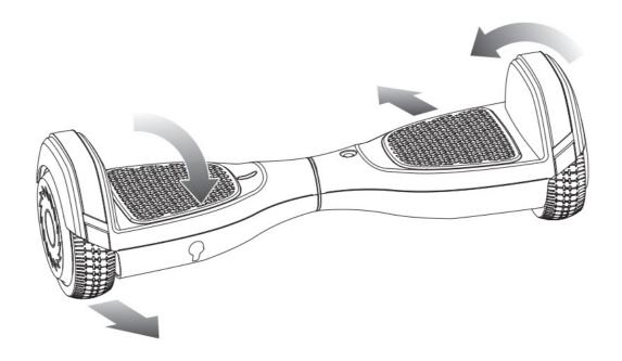
MOVEMENT OF THE RAZOR HOVERTRAX 2.0 IS CONTROLLED BY THE ANGLE OF THE FOOT PLATFORMS, WHICH IS DETERMINED BY PRESSURE APPLIED BY THE RIDER'S FEET ON THE PLATFORMS..
