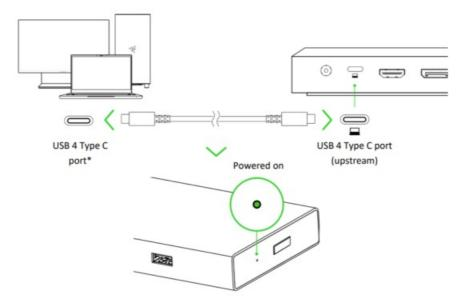
\*For optimal performance, it's recommended to connect the dock to a USB 4 Type C port. Please check your device's manufacturer for detailed USB device support.
