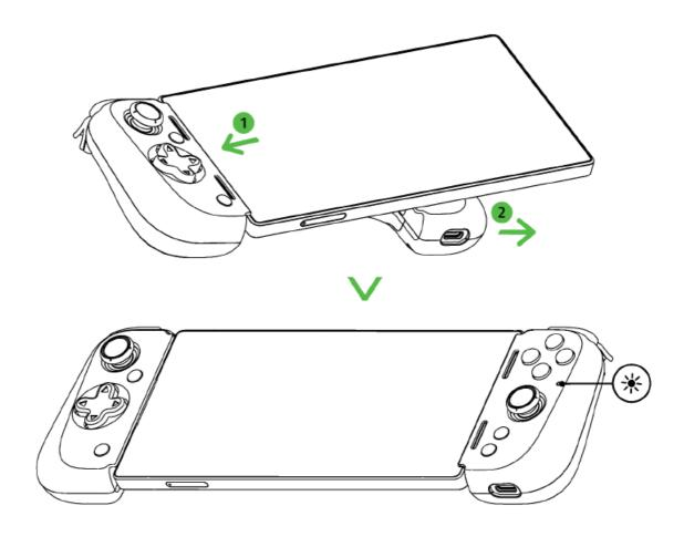
Maximum supported dimensions: 11.5 mm (thickness, including camera) x 170 mm (Length)
