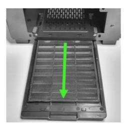
**Note:** Keep your chassis in optimal temperature by cleaning these dust filters as often as possible.
