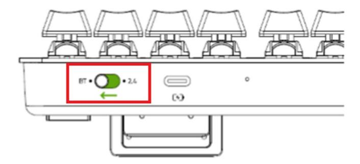
2. Up to 3 Bluetooth devices can be paired and registered to your keyboard (one for each profile). To activate the pairing mode of your preferred profile, press and hold its corresponding shortcut for 5 seconds. The LED indicators will then display which Profile has been activated.
