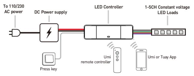
The controller supports 1-5 channel application from single color to RGB+CCT, please refer to following diagram for multiple application output wiring.
