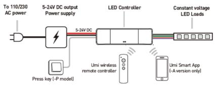
**Model NM40-**A supports 1-4 channel applications from single color to RGB+CCT, please refer to the following diagram for multiple application output wiring.
