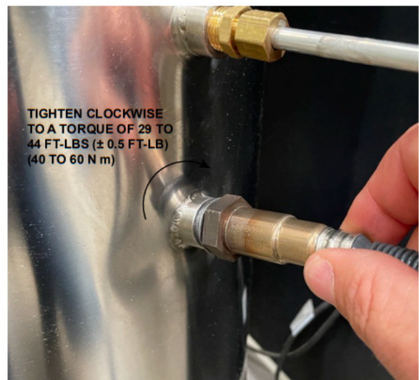
Figure 18. Installation of Oxygen Sensor
