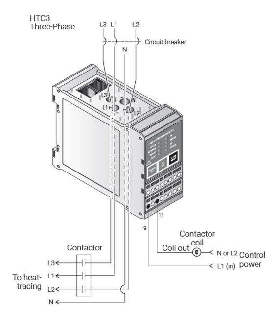
**WARNING:** Shock Hazard. Disconnect from live voltage prior to accessing terminals.
