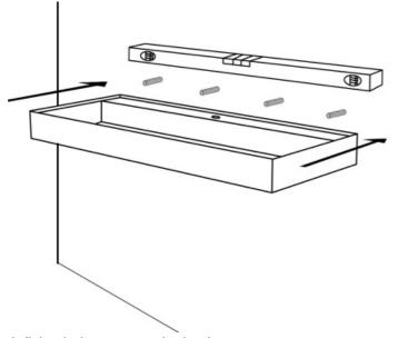
4. Screw a metal nut onto each fixing bolt to secure the basin.
