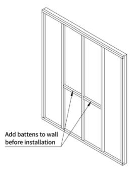
2. Important! Before installing, ensure there is sufficient timber framing in the wall to securely fasten your basin to.
