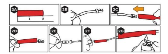
For the unused extension harness connectors (mentioned in the next step) cut 1.5" piece of heat shrink tubing, slide it over the connector and heat shrink it using a lighter or heat gun. Use needle nose pliers to pinch the end of the extra heat shrink. This will act as a cap to protect the connectors from getting dirt inside. [SEE FIGURES 2H – 2L]
