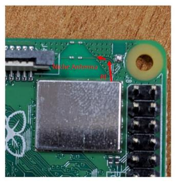
• Niche Antenna on board connected to the passive RF switch (Skyworks Part number SKY13351-378LF), switch directly connected to the Module. You must follow the design guidelines for the antenna.
