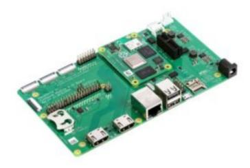
The Compute Module 4 IO Board is a companion board for Raspberry Pi
