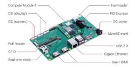
Input power: 12V input, +5V input with reduced functionality (power supply not supplied)
