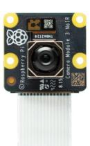
Raspberry Pi Camera Module 3 is a compact camera from Raspberry Pi. It offers an IMX708 12-megapixel sensor with HDR, and features phase detection autofocus. Camera Module 3 is available in standard and wide-angle variants, both of which are available with or without an infrared cut filter.
