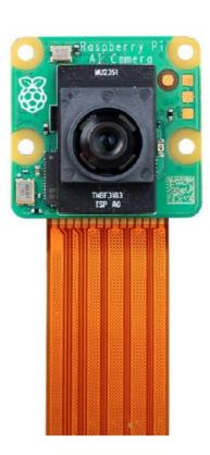
The Raspberry Pi Al Camera is a compact camera module from Raspberry Pi, based on the Sony IMX500 Intelligent Vision Sensor. IMX500 combines a 12-megapixel CMOS image sensor with on-board inferencing acceleration for a variety of common neural network models, enabling users to develop sophisticated vision-based Al applications without the need for a separate accelerator.
