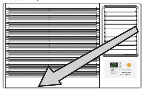
■ Occasionally there is the sound of "GI-GA", the expansion and contraction of the front leaf window due to temperature changes.
