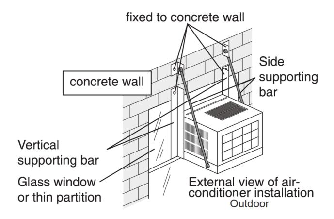
• Proposed to use 1/8" x 1-1/4" "angle-aluminium for installation frame and side supporting bar.
