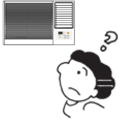
■ There seems to be a sound of running water. This is the sound of the refrigerant flowing inside the air conditioner.
