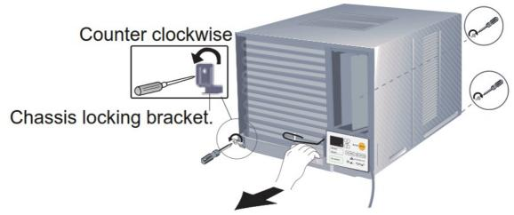
3. Place the cabinet into the installation hole.
