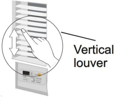
**NOTE:** Vertical adjustment of the airflow direction is done manually.
