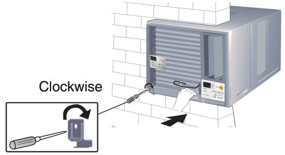
6. Depending upon the location of AC outlet, route the AC cord to either left or right side before Installing the front grille.
