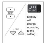
The temperature can be set between 16°C and 30°C.
