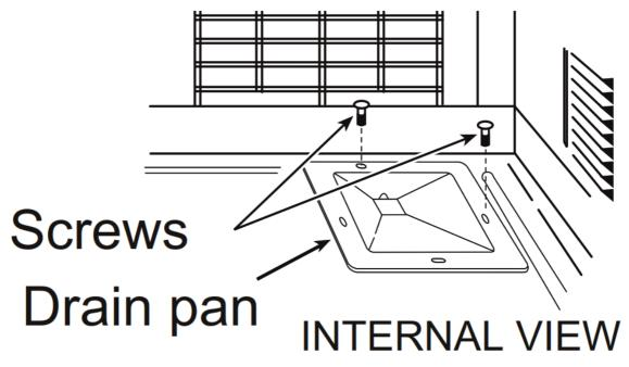
Install the drain pan at the right corner of the cabinet using 2 screws.
