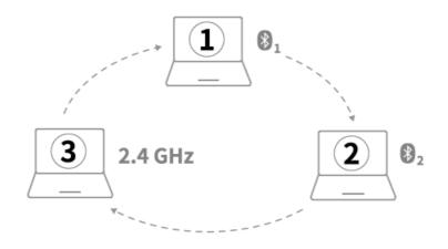
Press Bluetooth button to switch among up to 3 paired devices. Ihe mouse connects up to 2 devices Via Bluetooth and 1 Via a 2.4 GHZ receiver.
