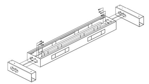
• Step 2: Install the U brackets to the desk frame with 4 pcs M8x10 screws. Mount the cable tray to the desk frame and fix it with 6 pcs M6x10 screws.
