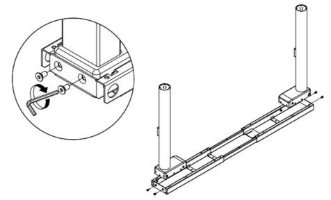
• Step 3: Place the table feet on the Column and rotate it to align, then tighten the preinstalled bolt.
