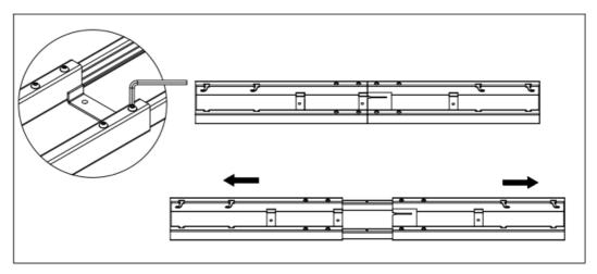
• Step 2: Insert the Column to the top frame, fix lifting column with 4pcs screws M6x12.
