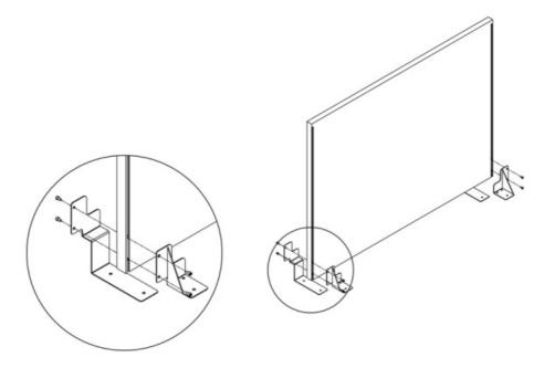
• Step 3: Fix the screen brackets (B2-SBRAC) to the desk frame with 10 pcs M6x10 screws.
