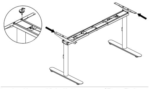
• Step 5: Mount the tabletop and fix it with 14 pcs screws ST4x20. Fix the centre bracket with 2 pcs screws M6x10. Tighten the pre-installed bolts on the top frame.
