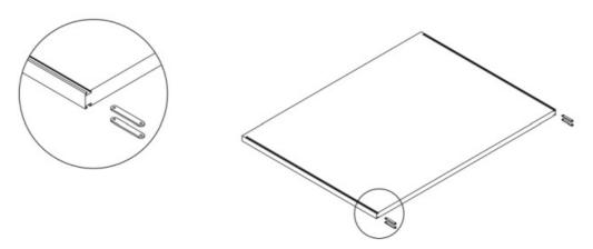
• Step 2: Install the screen brackets (B2-SBRAC) to the Shush30 Extrusion with 8 pcs M5x6 screws.
