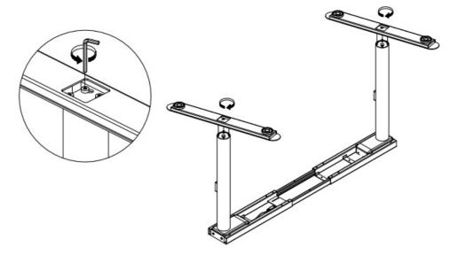
• Step 4: Place the side bracket on the top frame and tighten the bolts.
