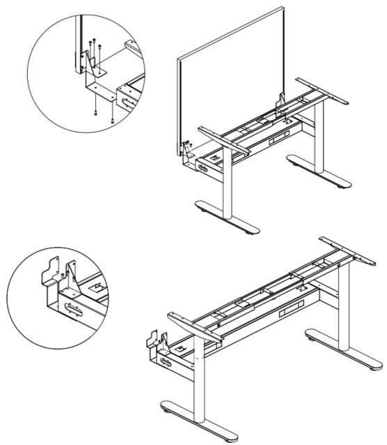
• Step 2: Place the EPS panel on the screen brackets. Using a 6mm drill bit (not included), drill out holes in Eco Panel Screen in line with back-to-back screen bracket holes. Place 8 x Double Ended Bolts M5\*32mm – 6mm through The screen bracket (B2-SBRAC) holes and the holes you have created in the Eco Panel Screen. Tighten double-ended bolt with Allen key.
