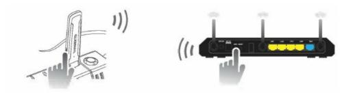
Tips: If you want to keep the stable connection between your router and our repeater at REPEATER mode, Please install our Repeater at a suitable position. You can check the suitable position as the followings: You can check the Wi-Fi signal on your smartphone, if the signal is below 2 levels, we suggest to change the location of our repeater.
