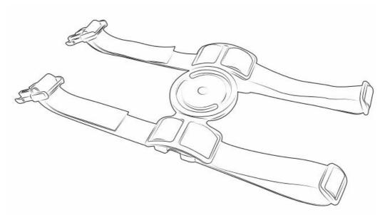
4. Route any excess strap back through the (A) Body Mount Base slots.
