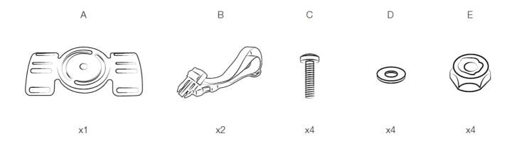
1. Remove male buckle from (B) Buckle Strap, and route through slots of (A) Body Mount Base as shown.
