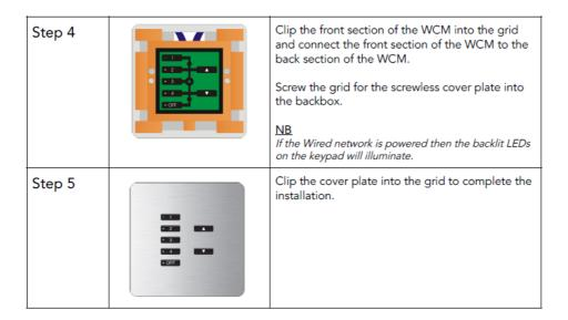
Installation of the WCM (Screwed plates)
