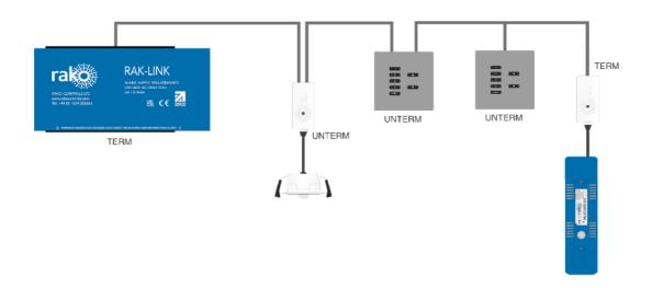
**STAR Wiring** A STAR Wired system has individual runs from one or more RAK-STAR units to the Wired Devices, every end of line in a STAR system should have the STAR termination.
