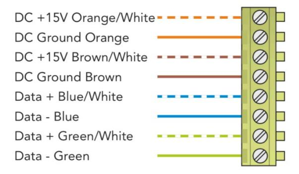
Used when the WCM-D is not at the end of line (with or without a RAK-STAR). This is usually identifiable by two cables being connected to the WCM-D.
