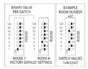
When power is initially connected to the module the unit should switch the load ON. The load can then be manually switched using the Set-up button under the top cover (see Fig.2 overleaf). The factory set address for both modules and transmitters is House 1 Room 4 (See Fig 1 for further information). A Rako wireless wall panel set as address House 1 Room 4 will control and dim the module. Should the module not respond as above then further investigation should be made before proceeding further.
