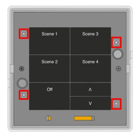
These must not be adjusted. Adjusting these may damage RK-MOD-xxx-x
