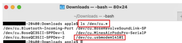
Figure 23: Checking the RAK4631 USB port connection
