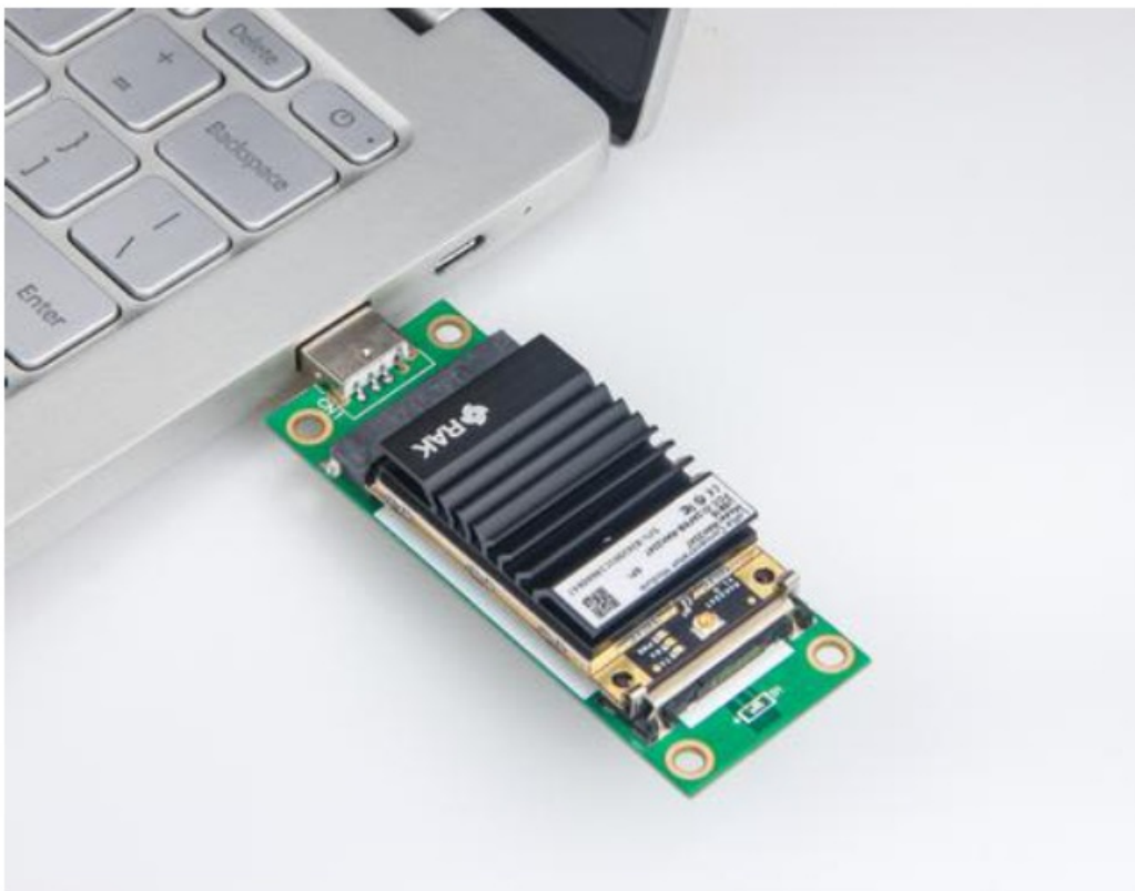
Figure 2: RAK2247 WisLink LPWAN Concentrator to a PCIe-to-USB board
